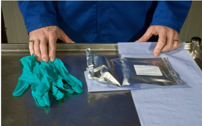
Open foil pack and remove test kit
